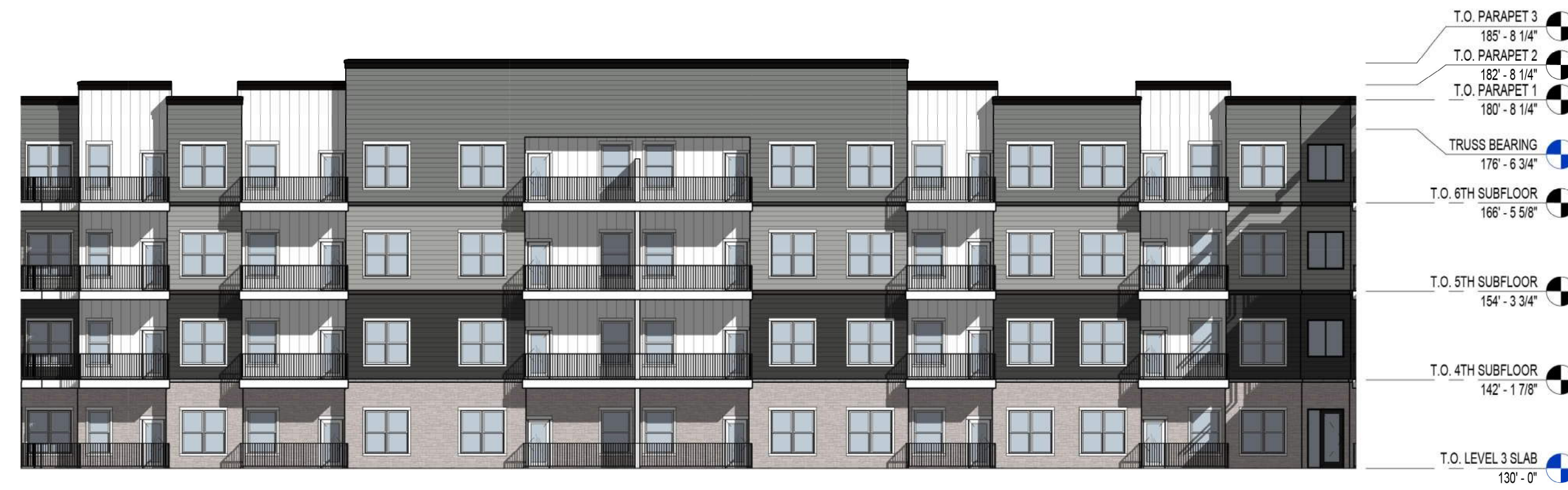
4 COURTYARD 1 - WEST ELEVATION 1/16" = 1'-0"
