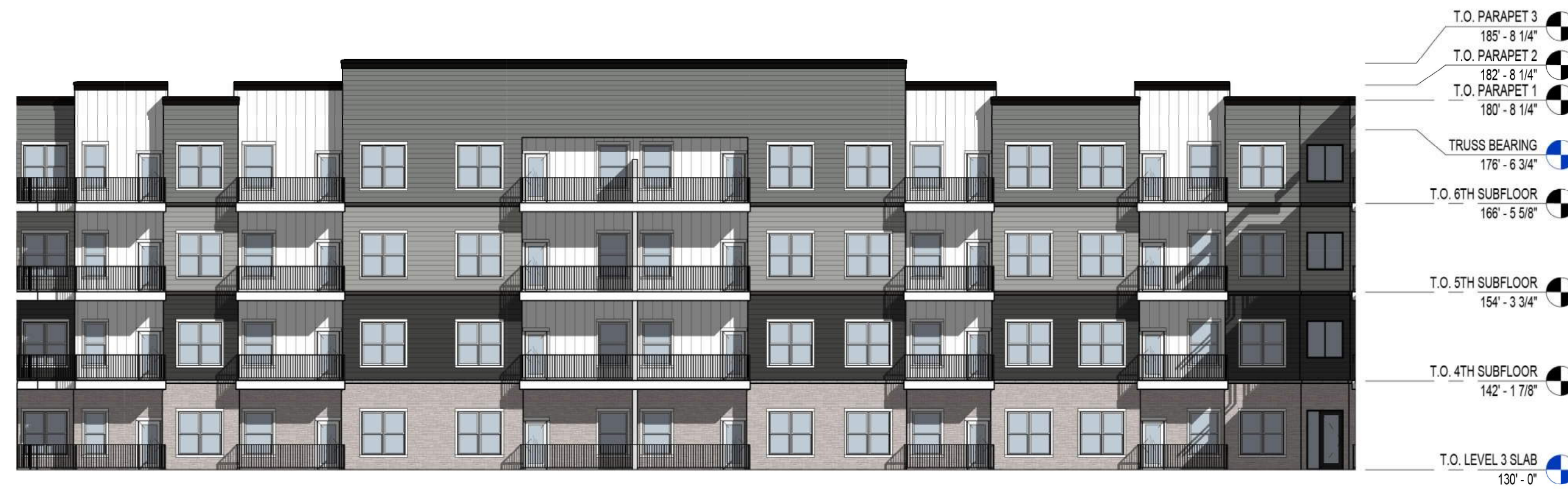
4 COURTYARD 1 - WEST ELEVATION 1/16" = 1'-0"
