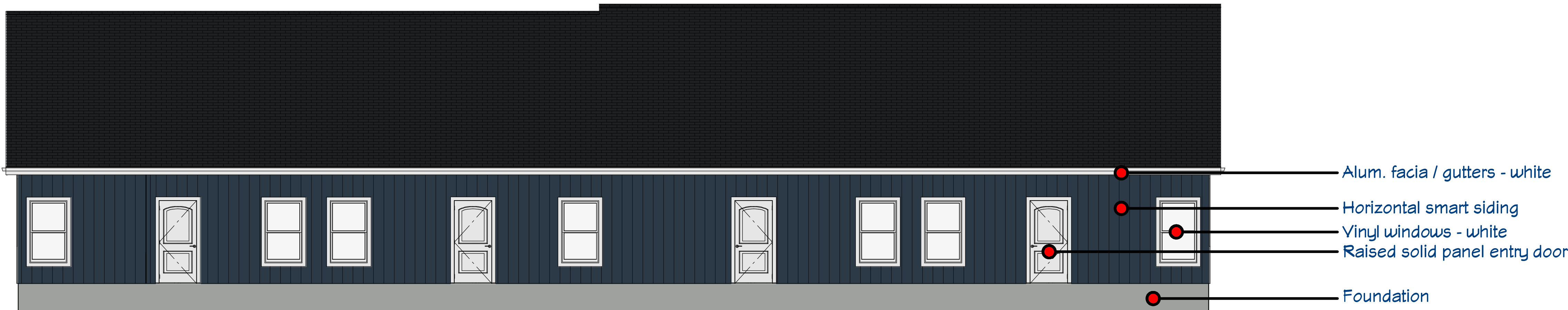
Exterior Elevation Rear
