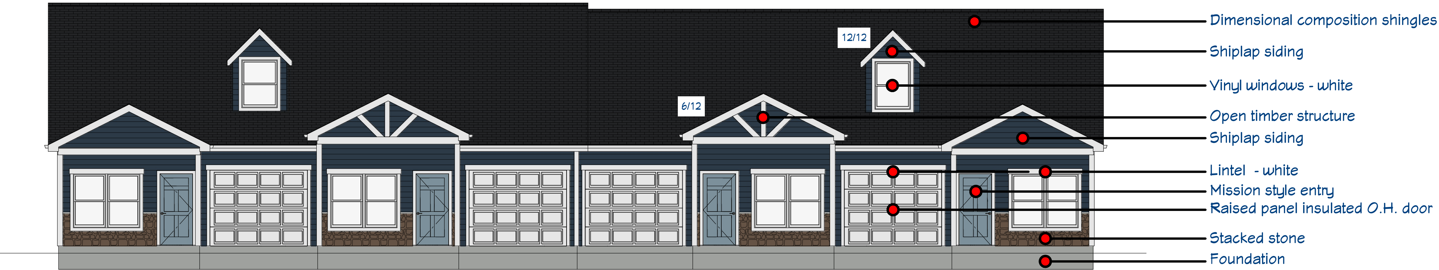
Exterior Elevation Front
