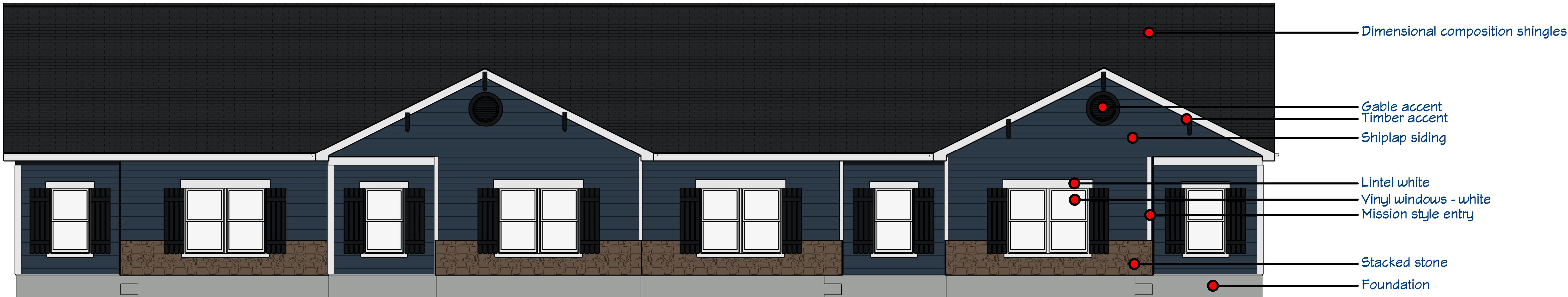
Exterior Elevation Front
