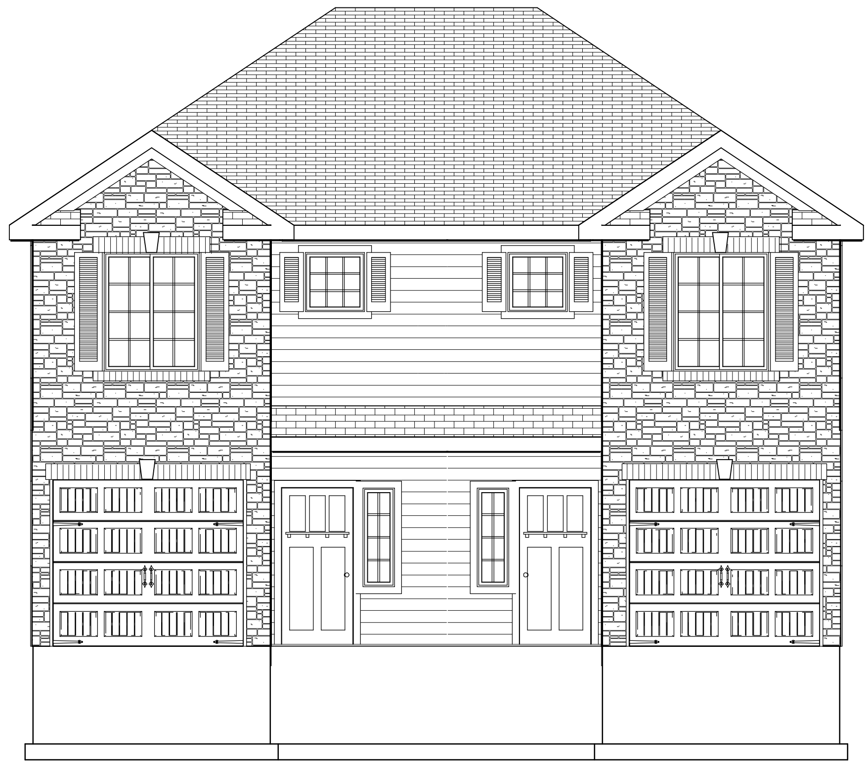
FRONT EL. VINYL SIDING AND STONE
