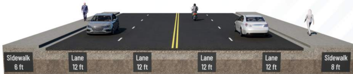
Off-Street Typical Section
