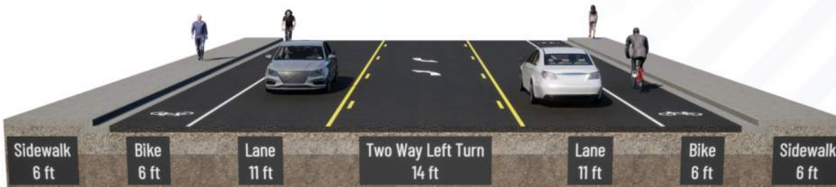
On-Street Typical Section
